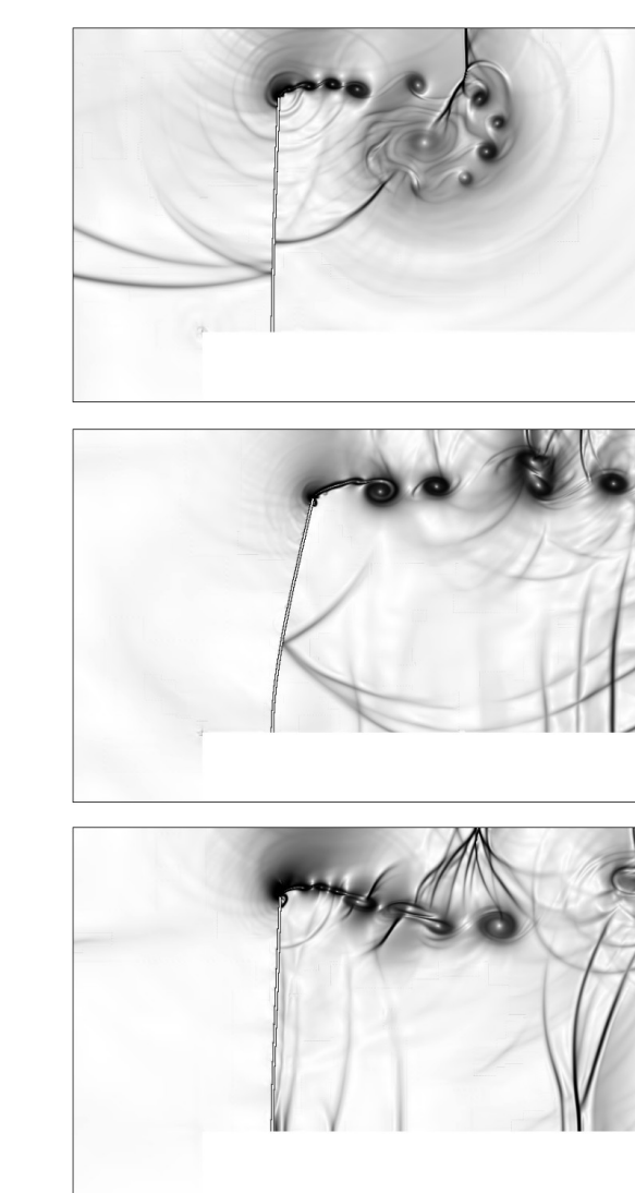
Right: Schlieren plot of fluid density in the vicinity of the thin steel panel. Snapshots for t=0.51\text{ms} , 1.63\text{ms} , and 3.02\text{ms} (from top to bottom). Vortex shedding from panel tip and beam vibration induced by shock impact.
