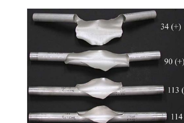
Top: Specimen geometry. Left: Typical experimental rupture patterns.
